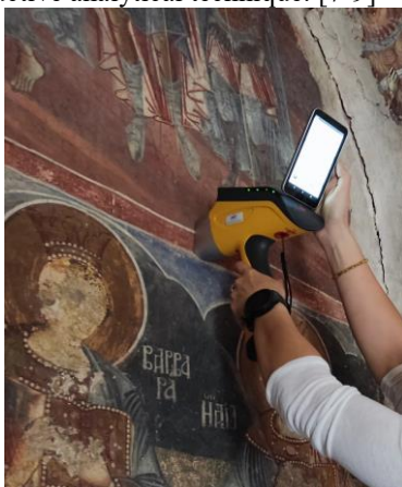
Fig. 2. Portable X-ray fluorescence (XRF) Explorer 5000 device.
