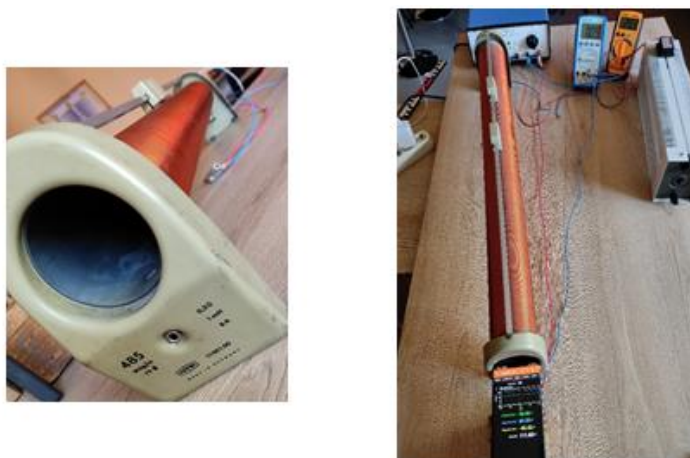
Fig. 11. Solenoid and scheme for the study of its magnetic field depending on the electric current
