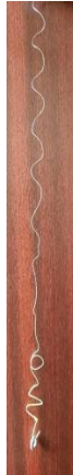
Fig. 3.4 - Small PLA spring using two materials with a small weight for analyzing the deforming parameters and quality of PLA different materials
