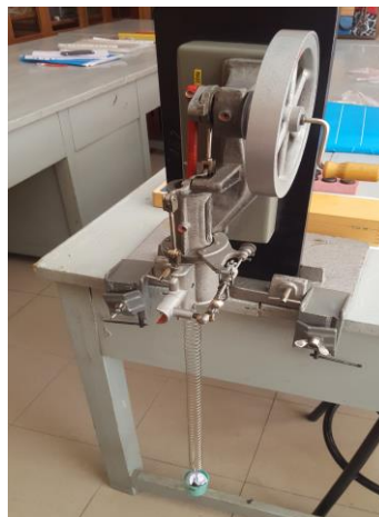
Fig. 5. The experimental setup that made it possible to realize forced oscillations.
