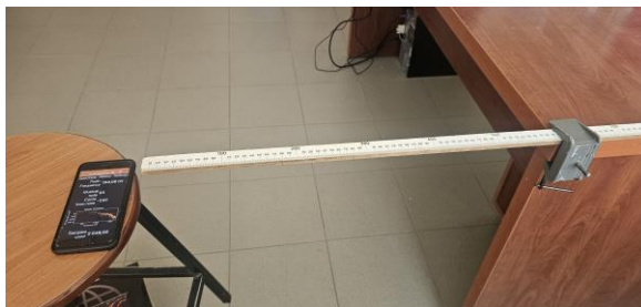
Fig. 4. A wooden rod of variable length, fixed at one end to the edge of a table, oscillates when displaced and released its free end.
