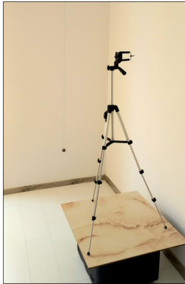
Figure 2. Experimental setup to record videos of simple pendulum motion.
