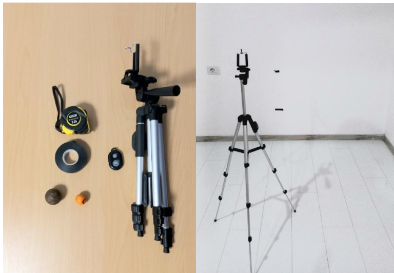
Figure 1. Experimental setup to determine acceleration due to gravity, g .
