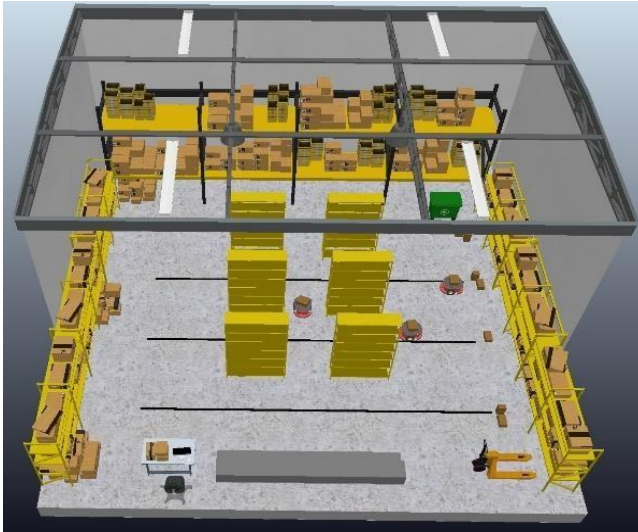
Fig. 2. CoppeliaSim warehouse simulation environment illustrating multi-tier storage racks, structured AGV pathways, docking stations, and dynamically generated package locations used for evaluating static and dynamic task allocation strategies.
