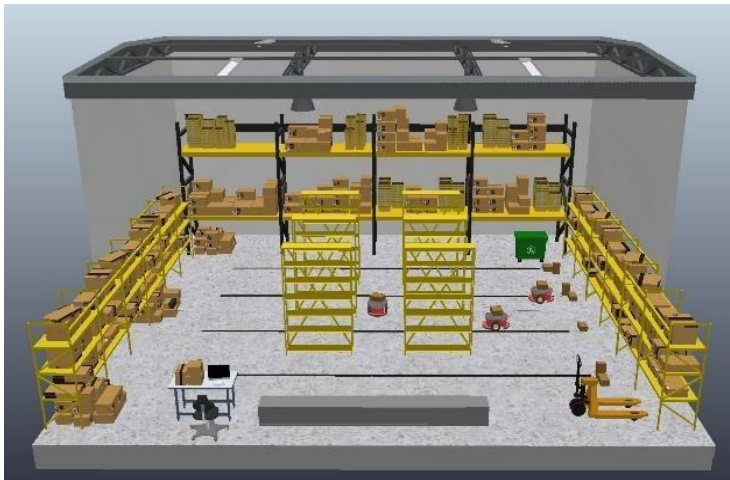
Fig. 2. CoppeliaSim warehouse simulation environment illustrating multi-tier storage racks, structured AGV pathways, docking stations, and dynamically generated package locations used for evaluating static and dynamic task allocation strategies.
