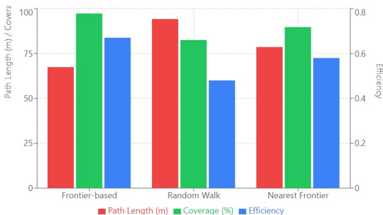
Figure 9. Path efficiency comparison: path length (in red), coverage percentage (in green), and efficiency ratio (in blue) for the three exploration strategies. The frontier based method achieves the optimal combination.
