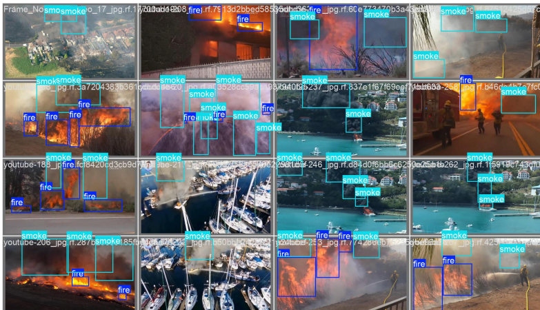
Figure 3. YOLOv8 fire and smoke detection results on test samples, the blue bounding boxes indicates fire and cyan bounding boxes indicates the smoke across diverse fire scenarios.
