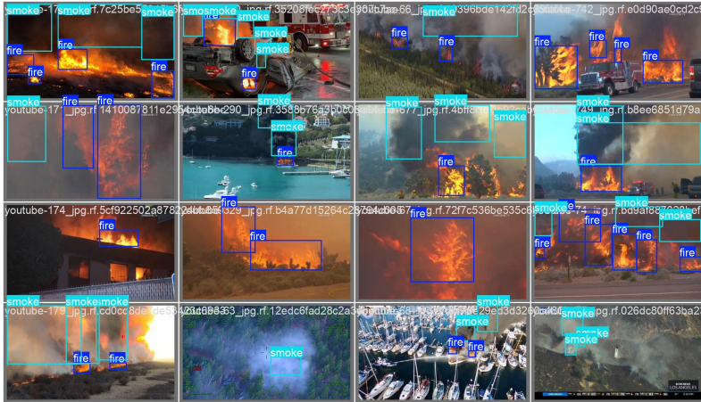
Figure 4. YOLOv8 detection results which demonstrates generalization across wildfire, structural fire, and smoke only scenarios.
