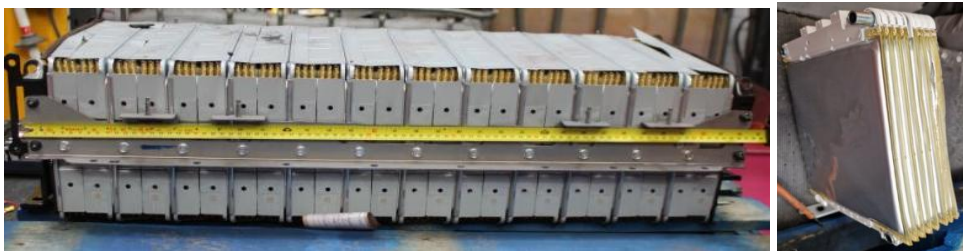
Fig. 6. Example of end-of-life Nissan Leaf battery modules and cells.
