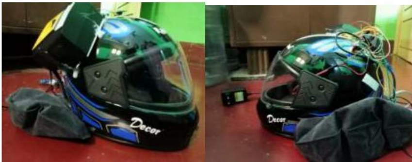
Fig. 1. Smart airbag with compressor [7]
