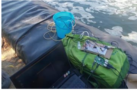
Fig. 8. Field Testing and Validation at ICAR-CIBA, Muttukkadu, Chennai. The prototype system comprises sensor modules integrated with a Raspberry Pi, collecting live readings from brackish water and transmitting data to a server for real-time monitoring.
