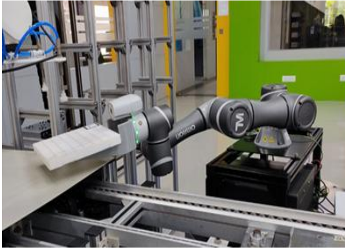
Fig. 10. Real-time execution of the “Place” command on the Omron TM5-700 cobot
