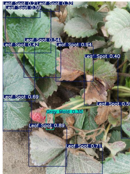
Fig. 8. Real-time detection system outputs showing identified diseases with bounding boxes and confidence scores for field application validation.
