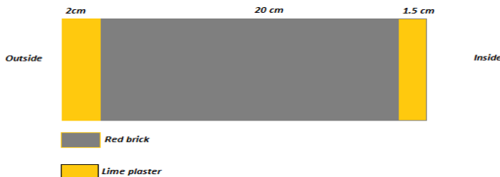
Fig. 5. Uninsulated red brick wall
