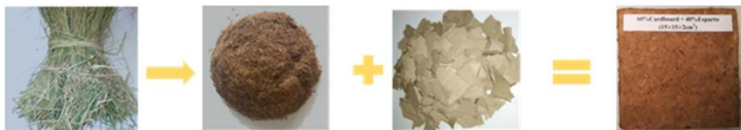
Fig. 2. Composite preparation using cardboard and esparto fiber.
