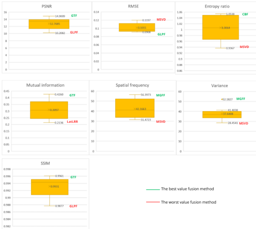
Fig. 6. Box plot representing the variation of metrics values per fusion method applied to the fused images
