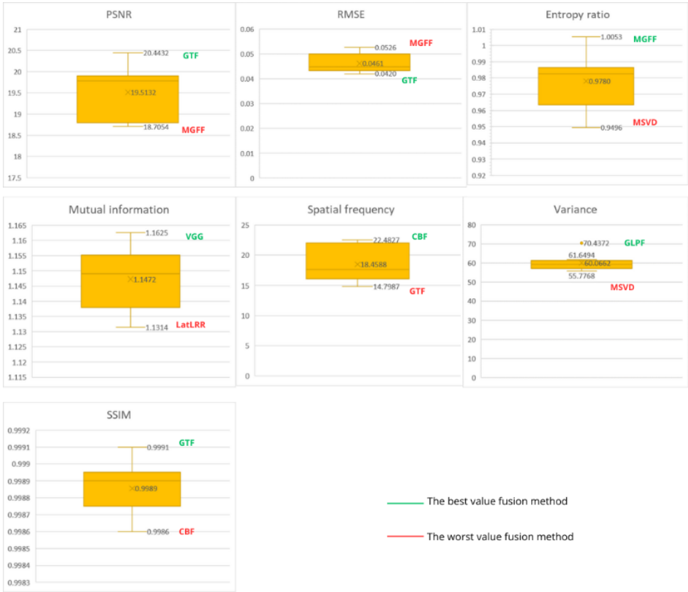
Fig.8. Box plot representing the variation of metrics values per fusion method applied to the target region (PV panel)
