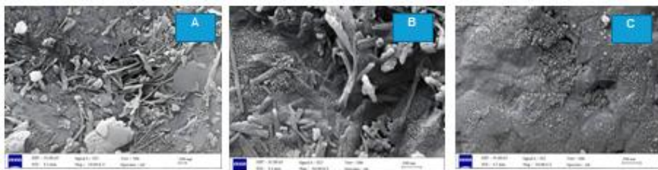
Fig. 6 SEM images for (a) virgin sand (b) coated sand (c) coated sand after interaction with Tetracycline antibiotic.
