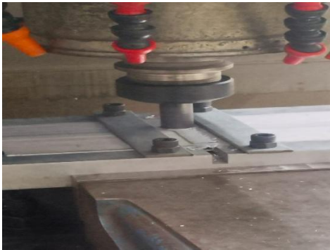
Fig.3(b). FSW joint preparation.
