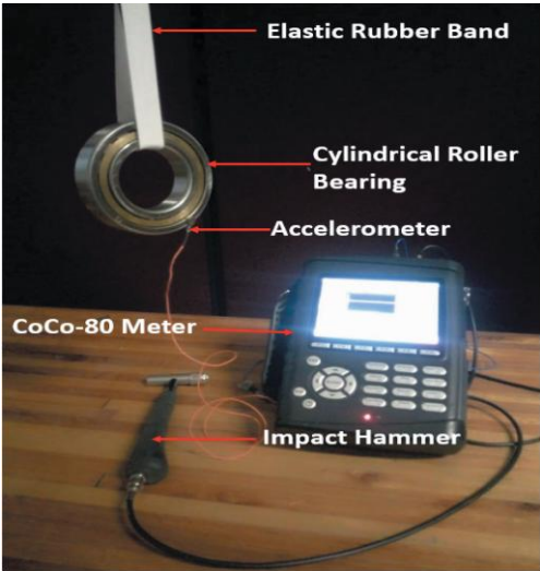
Figure 2. Experimental setup for frequency response testing [5]
