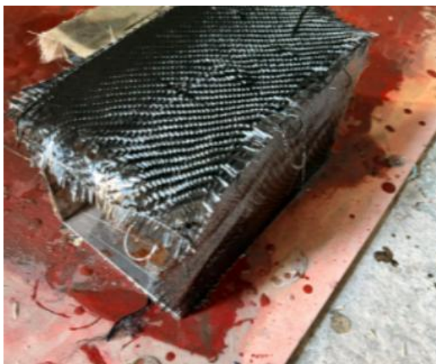
Fig. 18. Reinforced Part Using Carbon Fiber
