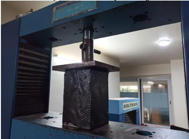
Fig. 39. Specimen under compression test using UTM.
