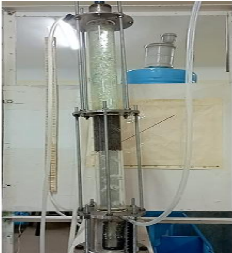
Fig 1. Experimental device of bubble absorber
