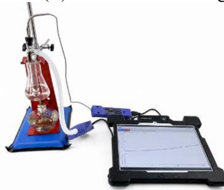
Fig. 2. Instrumental arrangement for gas heating in Gay-Lussac's Law testing
