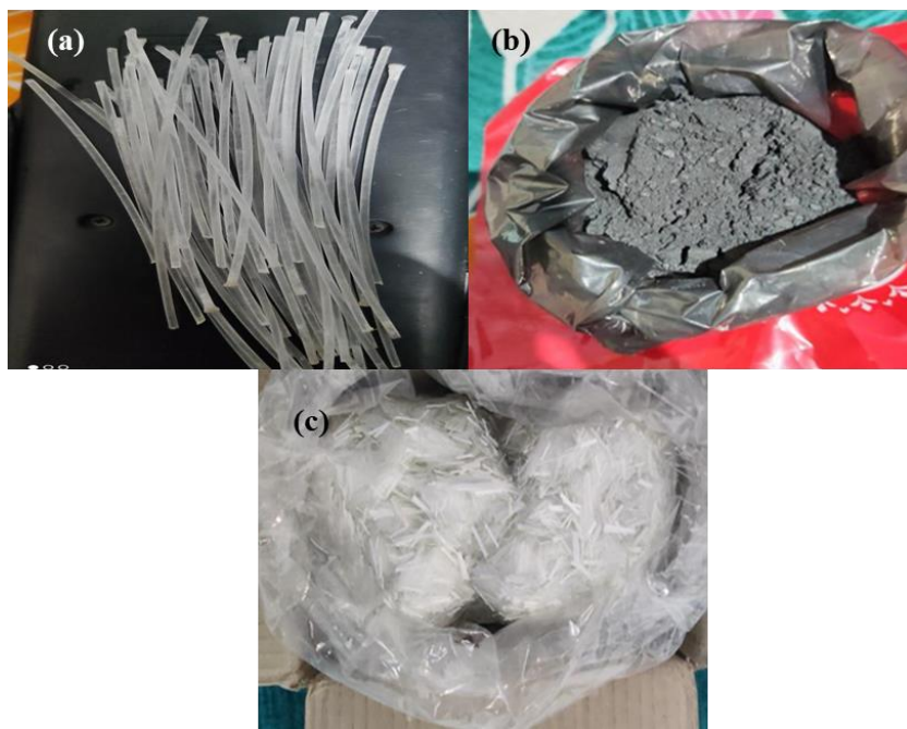
Fig. 1. (a) Optical fibers (b) Graphite powder (c) GF
