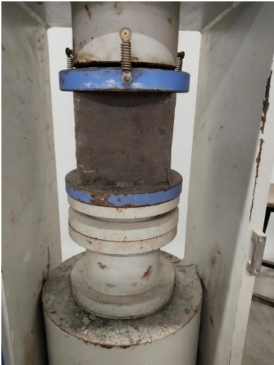
Fig. 1 Testing Sample for Compressive strength in Lab.
