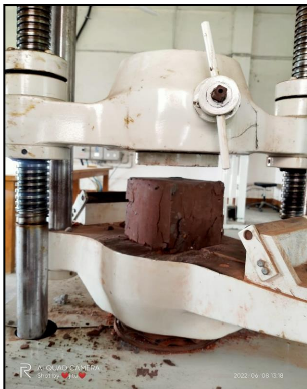
Fig. 4. Compressive Strength testing on Universal Testing Machine
