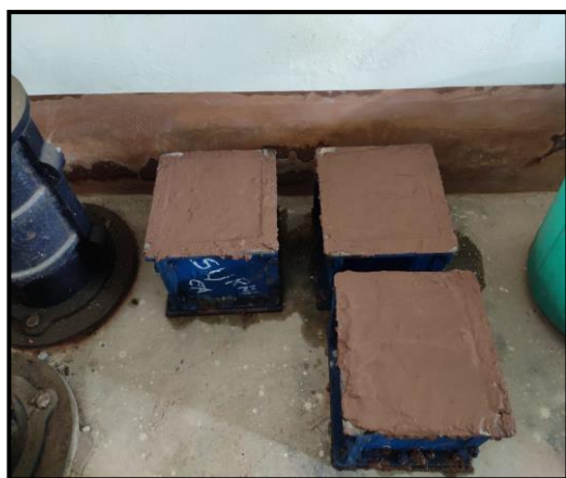
Fig. 3. Preparation of sample (fine aggregate replaced by surkhi)
