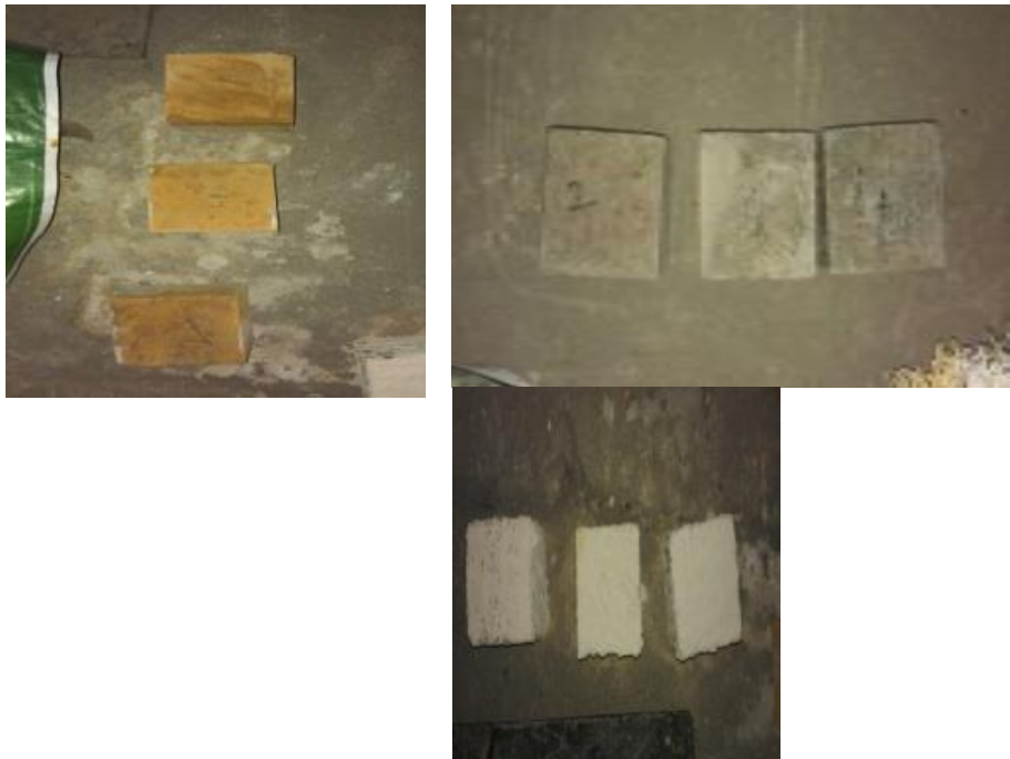
Fig. 5. Specimens of Processed Overburden Material Concrete after 28 days immersion in \text{H}_2\text{SO}_4 , \text{HCL} and \text{Na}_2\text{SO}_4 Solutions.
