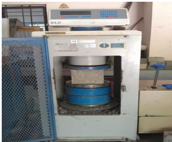
Fig. 2. Compressive strength of Processed Overburden Concrete specimen under testing.
