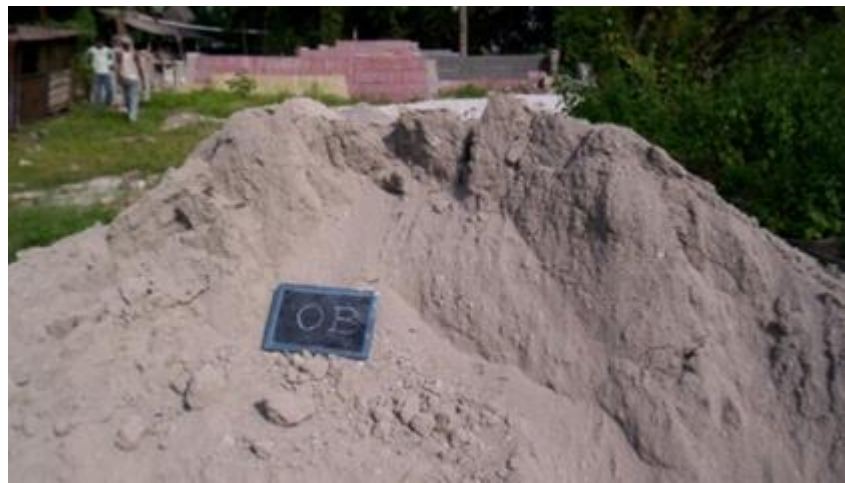
Fig. 1. Processed Overburden Material.
