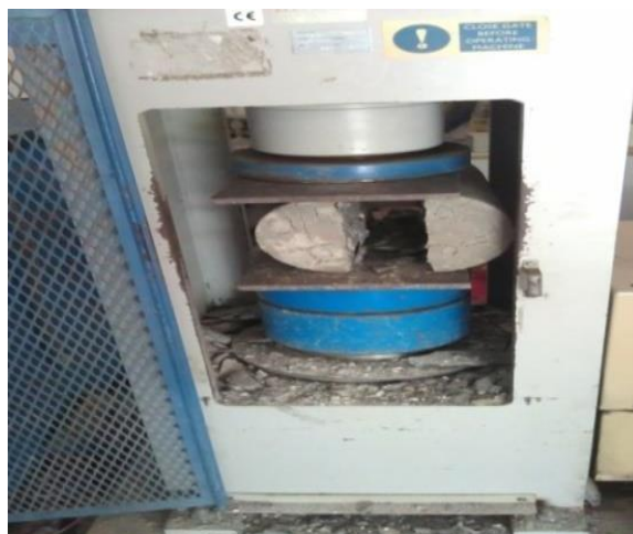
Fig. 3. Split Tensile strength of Processed Overburden Material Concrete specimen under testing.
