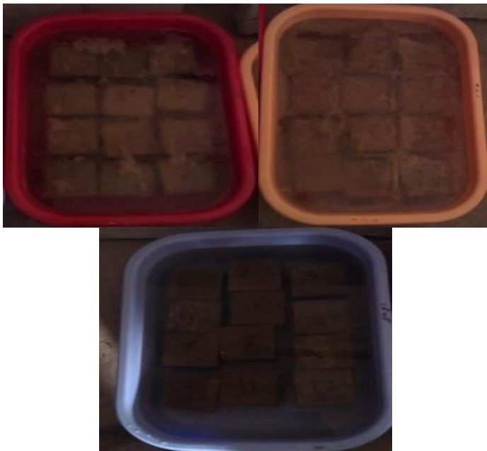
Fig. 4. Specimens under immersion for Durability test of Processed Overburden Material in \text{H}_2\text{SO}_4 , \text{HCL} & \text{Na}_2\text{SO}_4 Solutions.
