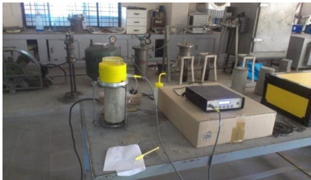
Fig. 6. Testing arrangements of water permeability test.
