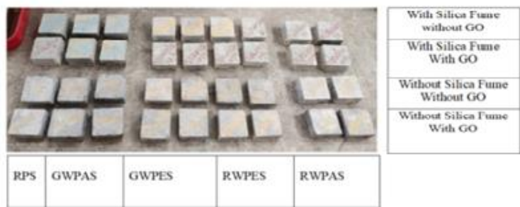
Fig. 1. Concrete cool roof slab panels after casting.
