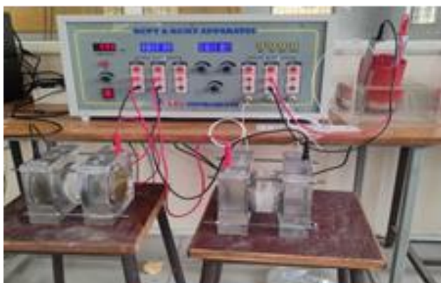
Fig. 3. Specimens under RCPT test
