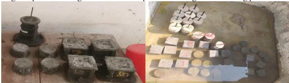
Fig. 2. Casting and curing of Specimen
