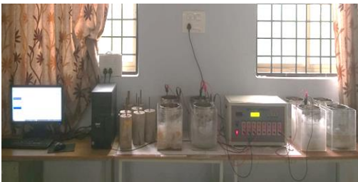
Fig. 15. Accelerated Corrosion Test
