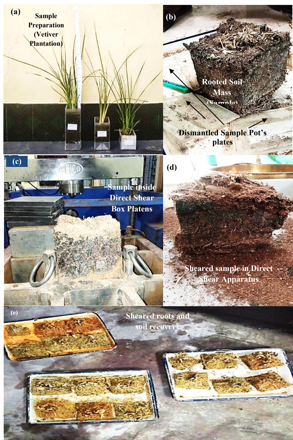
Fig. 2. Various Processes of the Direct Shear Test: (a & b) Sample Preparation with Roots, (c) Placement of Samples in the Shear Machine, (d) Sheared Sample, and (e) Recovery of Soil and Sheared Roots.
