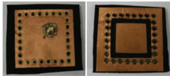
Fig. 9. Textile-based folded cavity-backed SIW antenna
